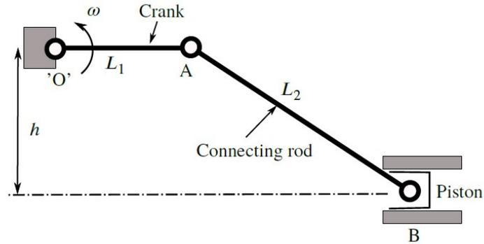
**Fig. 1:** Slider-crank mechanism
