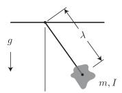
The pendulum pivots frictionlessly about a fixed point on the ceiling. The bob is fixed rigidly to the rod, which connects the pivot point to the bob's center of mass. Let m denote the bob's mass and I its rotational inertia with respect to its center of mass.
