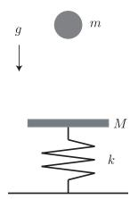
The ball drops a distance h before making contact with the platform, with which it collides with coefficient of restitution e. The system is aligned so that the ball and plate move only vertically as a result of the collision.
